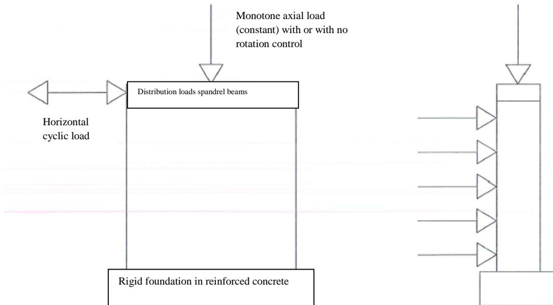
Figure 10-5: Tests type 5 (option) - Prototypes for experimental tests with combined application of actions in-plane and out-of-plane. Note that in the figure, the spandrel beams and the foundation elements have the only purpose of allowing the application of the load in testing phase; they are not an integral part of the structural element object of study
