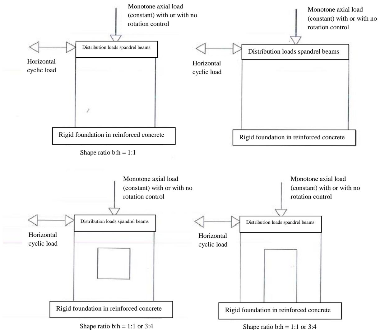
Figure 10-3: Type 3 tests - prototypes for experimental tests on full scale panels, on panels with no apertures ( $b:h=1:1$  e  $4:3$ ) with apertures ( $b:h=1:1$ ),  $h$  = storey height type, evaluation of strength, displacement capacity, dissipation. Note that in the figure, the spandrel beams and the foundation elements have the only purpose of allowing the application of the load in testing phase; they are not an integral part of the structural element object of study.
