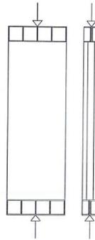
Figure 10-2: Type 2 tests - full scale panel prototypes (abt.  $h$ = storey height type,  $b > 1.0$  m), evaluation of collapse load for local and global panel instability
