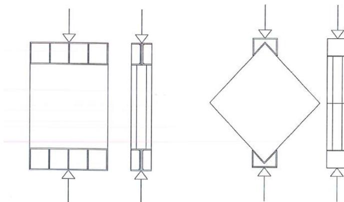
Figure 10-1: Type 1 tests - small size prototypes (abt. 1.0 m x 1.0 m), calculation of the modulus of elasticity
