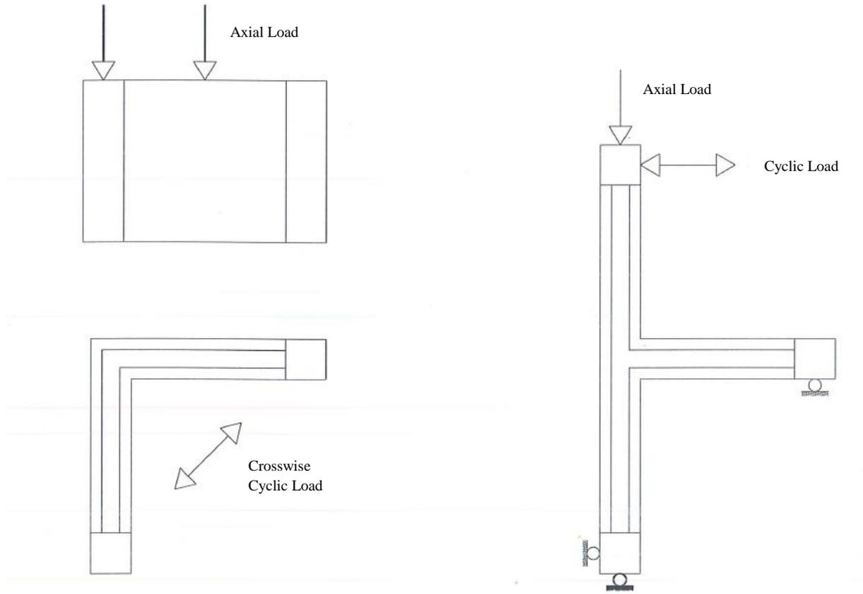
Figure 10-4: Tests type 4 - Prototypes for experimental tests on L and T shaped connections.
